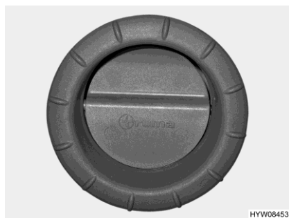
Fig. 79 Air outlet nozzle (hot-air heater)
