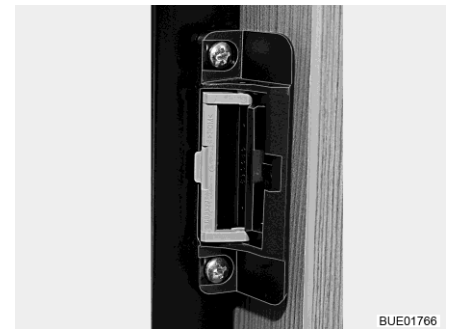
Fig. 90 Locking device in ventilation position
