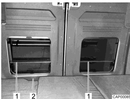
Fig. 40 Fall out protection (longitudinal rear bed)
