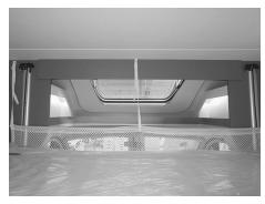
Fig. 127: Lowered lift-up bed with net to prevent falling out
