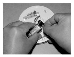
Fig. 162: Replacing the block battery
