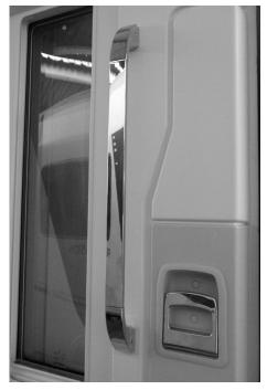
Fig. 17 Interior door with grab bar and handle, example
