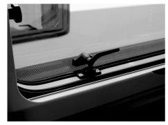
Fig. 88: Continuous ventilation
