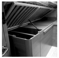
Fig. 42: Gas pressure spring
