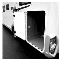
Fig. 18: Service compartment on the outside of the caravan; example: Small storage compartment for frequently used vehicle tools and travel equipment
