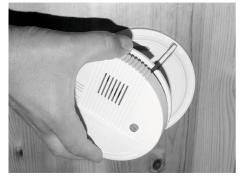
Fig. 161: Removing the housing
