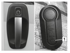
Fig. 10: Door handle, key with remote control for the central locking system
