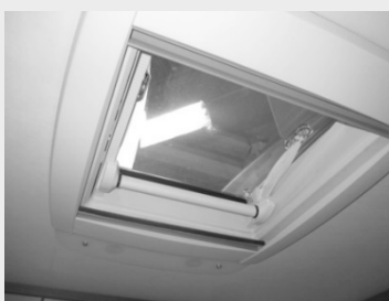
Fig. 35: Oblò 400x400 mm VisionStar 700x500 mm
