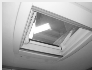
Abb. 36: Dachhaube 400x400 mm VisionStar 700x500 mm
