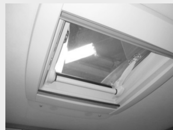
Abb. 22: Dachhaube 400x400 mm VisionStar 700x500 mm
